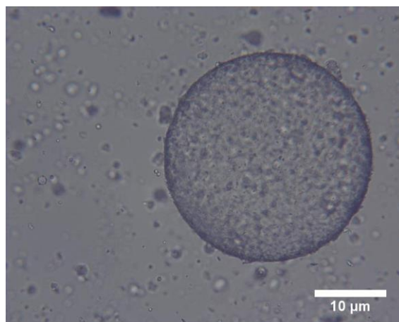
Figure 4.28. Example of the arrangement of fine CaSt 2 particles on the interface
