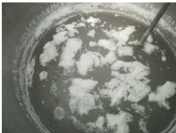
Figure 4.33. BR particles after their formation in the “flash drum” (W/O emulsion: organic phase: 50 g/L BR, aqueous phase: 0.1 M NaOH and 15 g/L CaSt 2 ).
