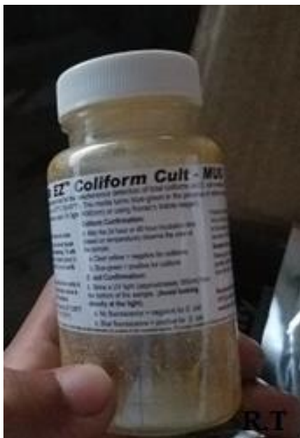
Coliform presence test kit allowing the detection of eventual faecal contamination of water
