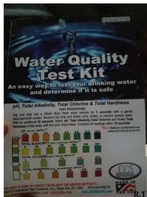
Water quality test kit used by MWP team allowing to determine the chemical composition of water
